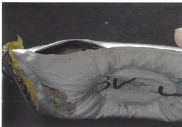
Figure 5. Pouch cells after punching test
